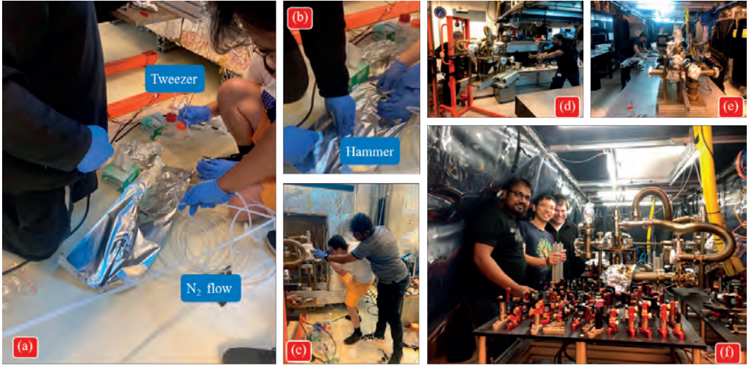
FIGURE 4.4: Loading strontium and moving the machine back after the bake. (a)-(c) Loading strontium from the glass cell into the oven reservoir. (d)-(f) Moving the machine to the lab and building up the Boikon framework it sits on.
