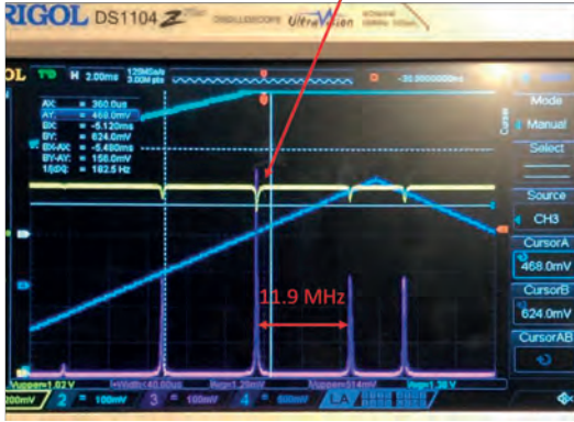
FIGURE 4.30: Example cavity finesse measurements. The sideband measurement of the linewidth of the transition peak using the well-known modulation frequency as the reference. Another method was ringdown measurement. The cavity was locked and once the input laser was turned off, the decay time from the output shows how many rounds photons bounce in the cavity, giving the finesse of the cavity.
