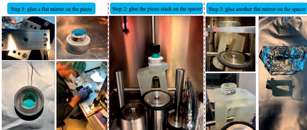
FIGURE 4.26: Processes of gluing flat mirrors. One flat mirror was glued on the piezo stack with a structure to protect the mirror from moving when the glue was curing in the oven. Then the piezo stack and another flat mirror were glued on the cavity spacer. The wires to the piezo stack were shorted and covered with aluminum foil.
