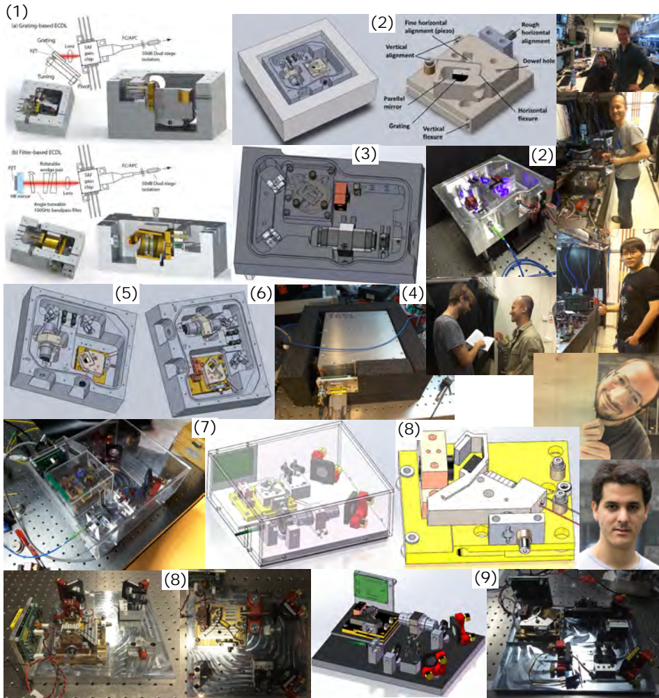
FIGURE 3.45: Evolution of the external cavity diode lasers (ECDLs) produced to run the SrCAL machine. (1) First designs - filter and Littrow ECDL designs from [300]. (2) First edition 461 nm master laser. (3) An alternate flexure design we considered as a first laser but never built. Before the first edition had been tested, we needed to make ECDLs for transparency and repump lasers so the first edition was just duplicated. For this reason the initial design lingered longer than it should have. (4) 688 nm transparency. (5) 707 nm with improved tuning adjustment. (6) 679 nm repump with diode separated from the housing and housing sealed to get below dew point. (7) 461 nm upgraded master without the large housing, on a simple baseplate improving accessibility and manufacturability (8) 448 nm repump with shorter cavity length and ideal pivot point. (9) 487 nm transparency with longer isolator and including an onboard AOM.
