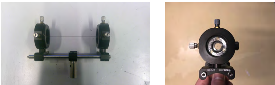
FIGURE 6.4: Dark cylinder. The dark cylinder used to block the MOT light from the transport dipole trap. Shown is the test unit rather than the final unit, which was similar but more than twice as long and constructed using a Thorlabs 30 mm cage frame and CXY1 mounts. The suspended capillary in the actual system is 200 mm long with a 600 \mu\text{m} diameter.
